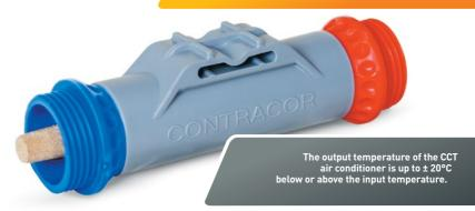
The CCT breathing air conditioner is designed for use with all blast helmets Comfort, Aspect, Commander and Panorama. It functions according to the principle of airflow separation and intended for heating or cooling breathing air which travels from the breathing air filter to the blast helmets.
