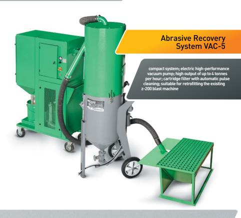
The VAC-5 abrasive recovery system is an electrically powered vacuum suction unit with an integrated high-performance cartridge filter comprising pulse-jet cleaning, an abrasive storage silo (mounted directly on the Contracor Z-200 series blast machine) for automatically refilling the blast machine and a floor hopper, complete with suction hoses and a grating.
