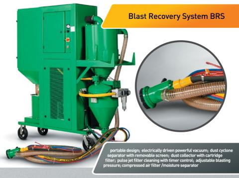
Closed-circuit abrasive blast cleaning, ideal for indoor blasting where dust and abrasive contaminants should be avoided, for the blasting of welding seams and for spot repairs. Used blast media are recyclable non-metallic media: glass bead, aluminum oxide (corundum).
